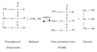
Fig. 1. A schematic representation of the transesterification of triglycerides (vegetable oil) with methanol to produce fatty acid methyl esters (biodiesel).
